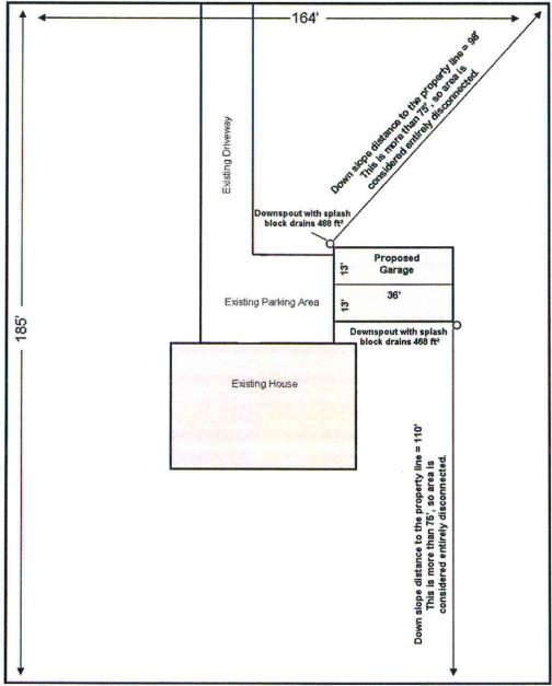
**Step 1:** Determine the area to each disconnected discharge. The area draining to each downspout is 468 ft<sup>2</sup>. This is less than 500 ft<sup>2</sup>, proceed to step 2.
